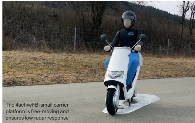
The 4activeFB-small carrier platform is free-moving and ensures low radar response
