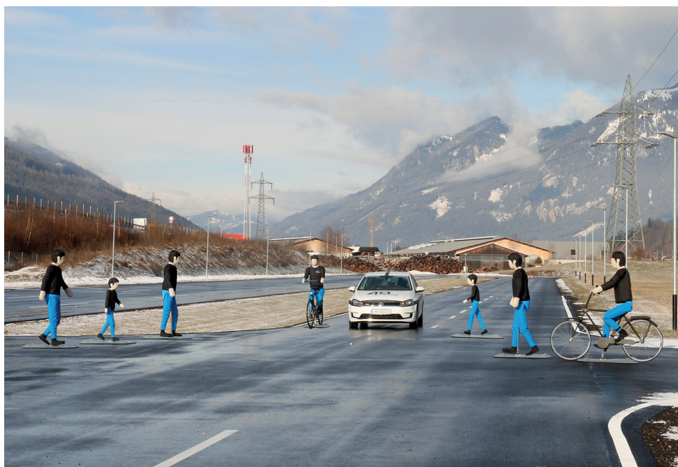
The free-moving platforms from 4activeSystems can be supplied with various dummy objects such as pedestrians or cyclists
